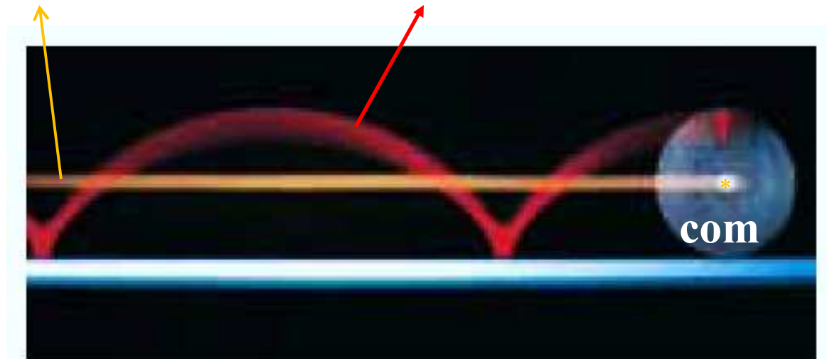
Fig. 11-2 A time-exposure photograph of a rolling disk. Small lights have been attached to the disk, one at its center and one at its edge. The latter traces out a curve called a cycloid. (Richard Megna/Fundamental Photographs)
