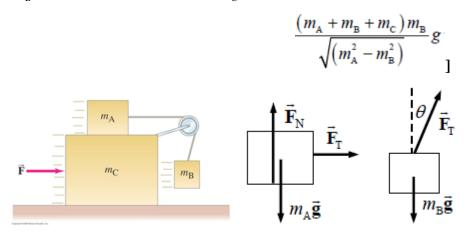
10) \*\*\* A 1.5-kg block rests on top of a 7.5-kg block (Fig. 4–63). The cord and pulley have negligible mass, and there is no significant friction anywhere. (*a*) What force *F* must be applied to the bottom block so the top block accelerates to the right at 2.5 m/s<sup>2</sup>? (*b*) What is the tension in the connecting cord? [Answer: a) 23 N, b) 3.8 N]
